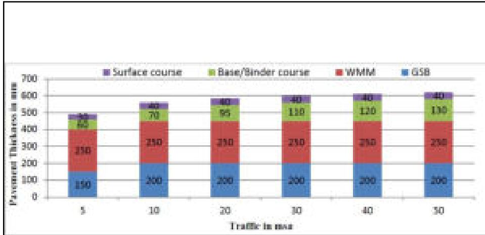
Figure 12.2 Catalogue for pavement with bituminous surface course with granular base and sub-base - Effective CBR 6% (Plate-2)
