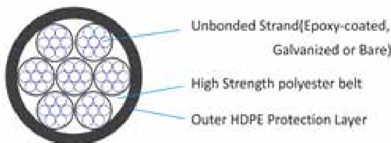
Fig: 7. 1 Prefabricated Cable GJ 15-7
