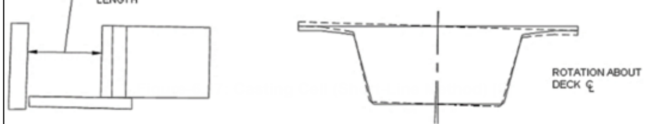
Figure-6.18: Form Adjustment in Casting Cell (Short-Line Method) [1]
