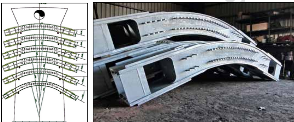
Fig 9.13 Upper Pylon with Saddle To Connect Stay Cable on both of its sides (Left), Fabricated saddle to anchor stay cable (Right)- Barapullah Extradosed Bridge Over River Yamuna
