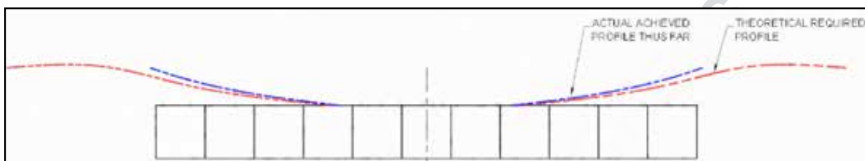
Figure-6.28 (a): Shimming Joints to Correct a Profile during erection [1]
