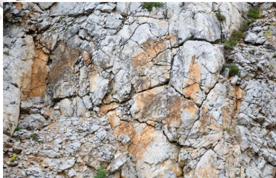
Stylolitic discontinuity with high shear resistance
