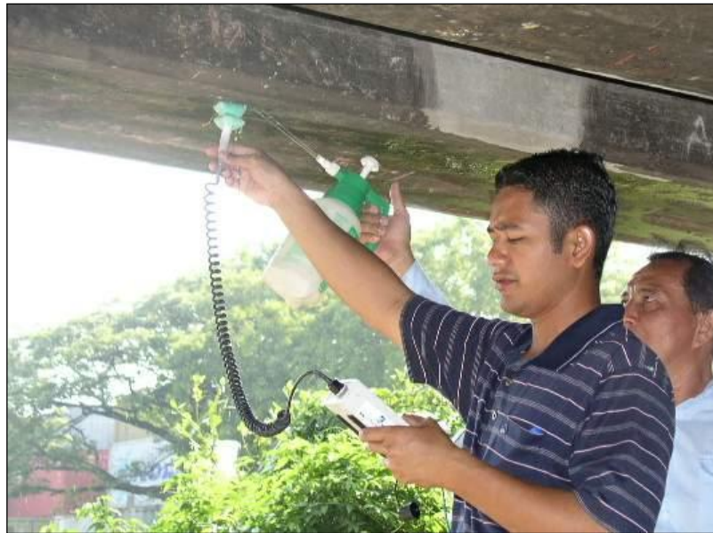
Figure 10.3: Placing the half-cell probe on the concrete surface
