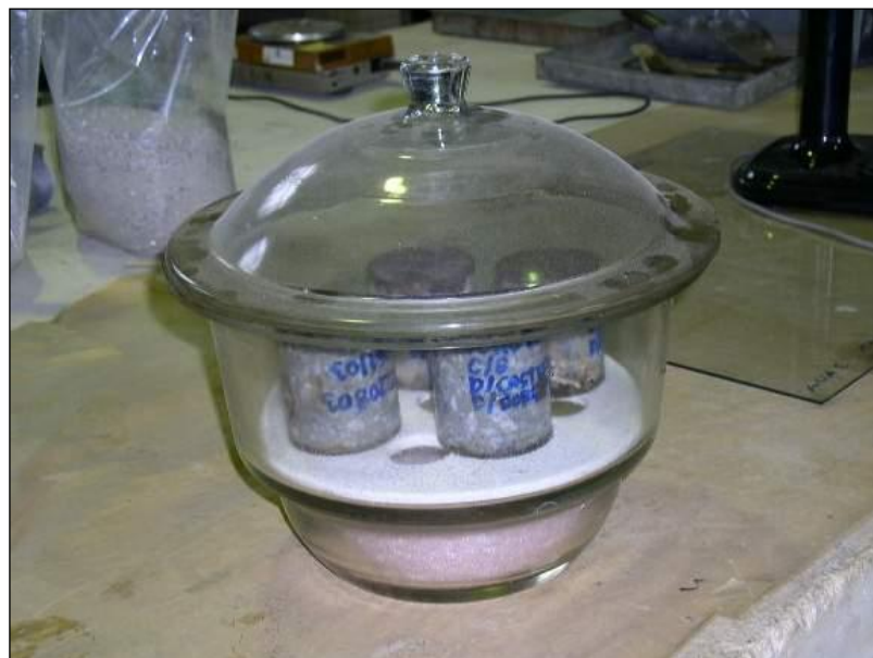
Figure 13.6: Storing specimens in a desiccator
