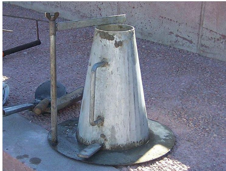
Figure 2.2: Slump cone and mixing pan
