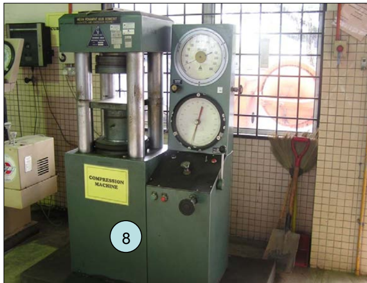
Figure 3.2: Cube compression test machine
