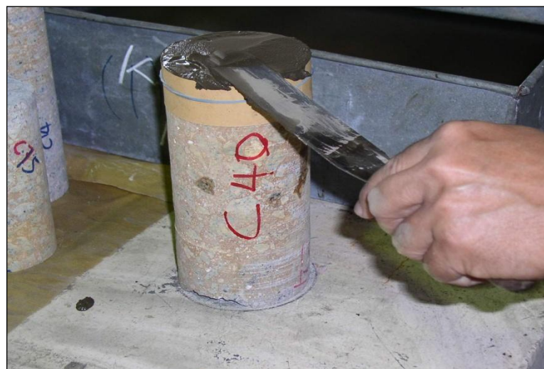
Figure 5.6: Capping the ends of specimen
