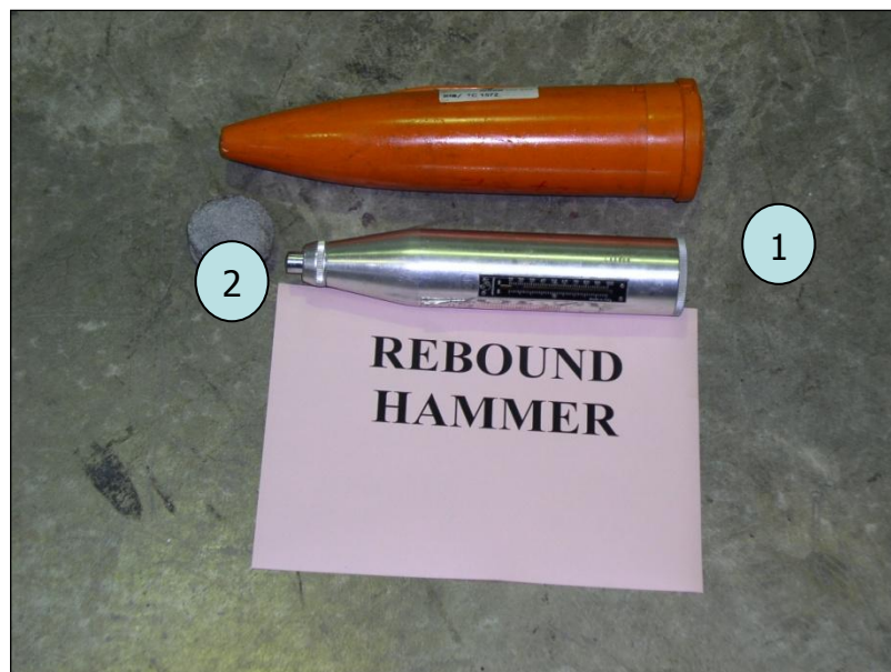
Figure 6.1: Rebound hammer apparatus
