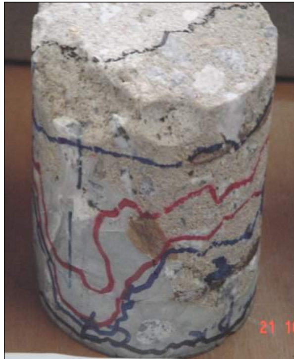
Figure 14.7: Draw water rising profile on specimen surface
