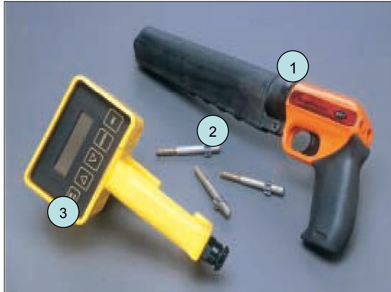
Figure 8.1: Windsor Probe test apparatus
