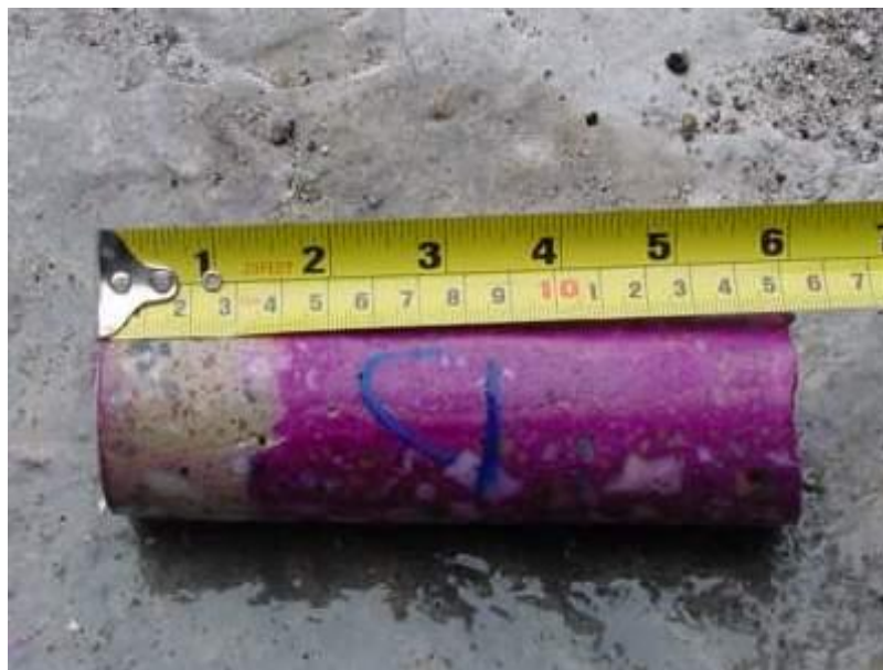
Figure 9.4: Measuring the carbonation depth of a core sample
