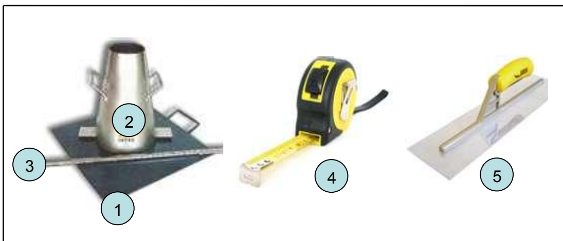
Figure 2.1: Slump test apparatus
