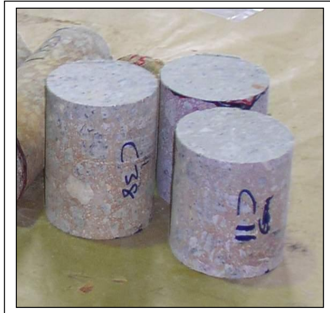
Figure 13.5: Cylinder specimens ready for water absorption test
