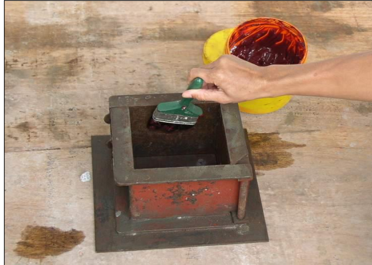
Figure 3.4: Applying grease to internal surfaces of mould
