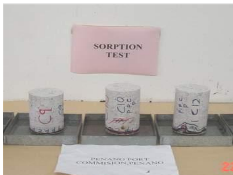
Figure 14.6: Placing specimens on the tray with water at 1-2mm height
