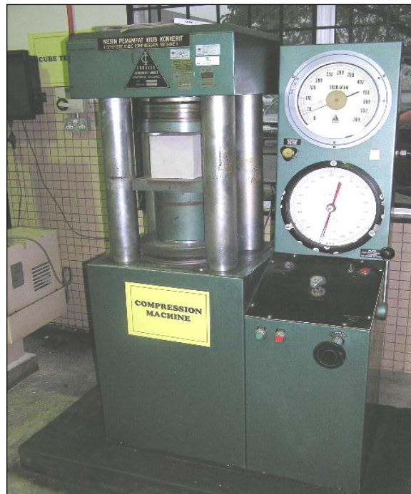
Figure 3.8: Testing for cube compressive strength
