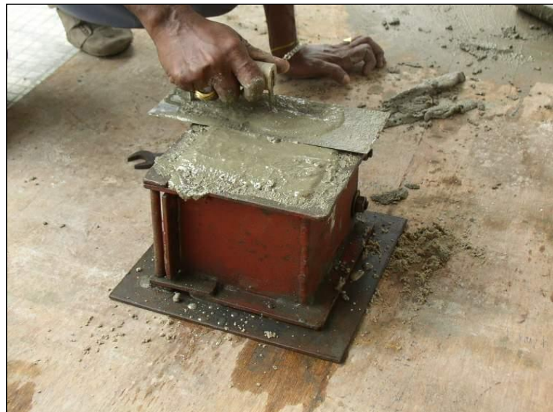
Figure 3.6: Levelling of mould surface with a plasterer's float
