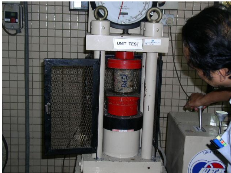
Figure 5.8: Testing for core compressive strength
