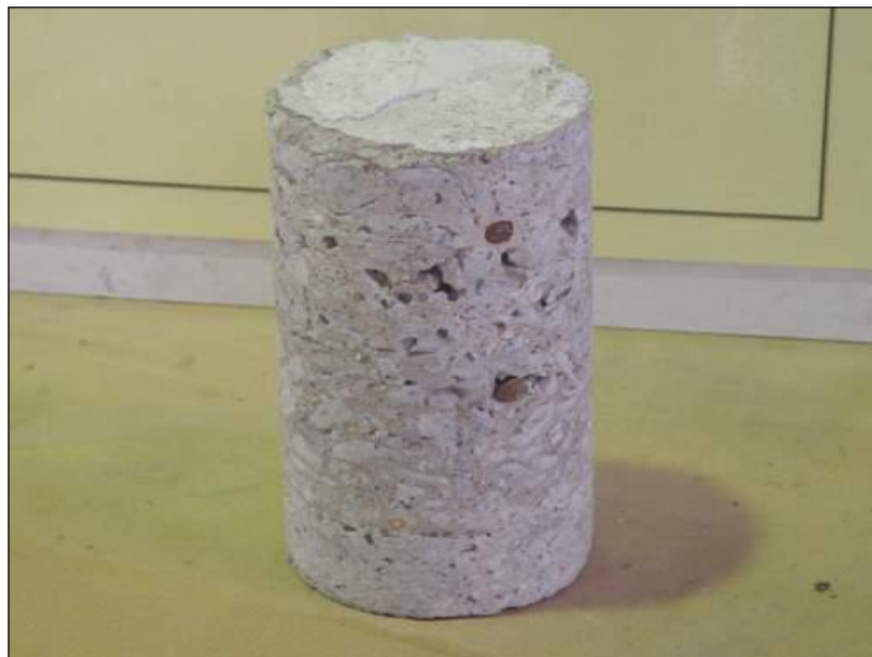
Figure 14.4: Specimen ready for sorption test
