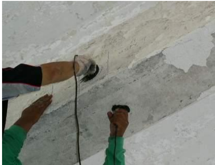
Figure 7.4: Arrangement of transducers for semi-direct transmission
