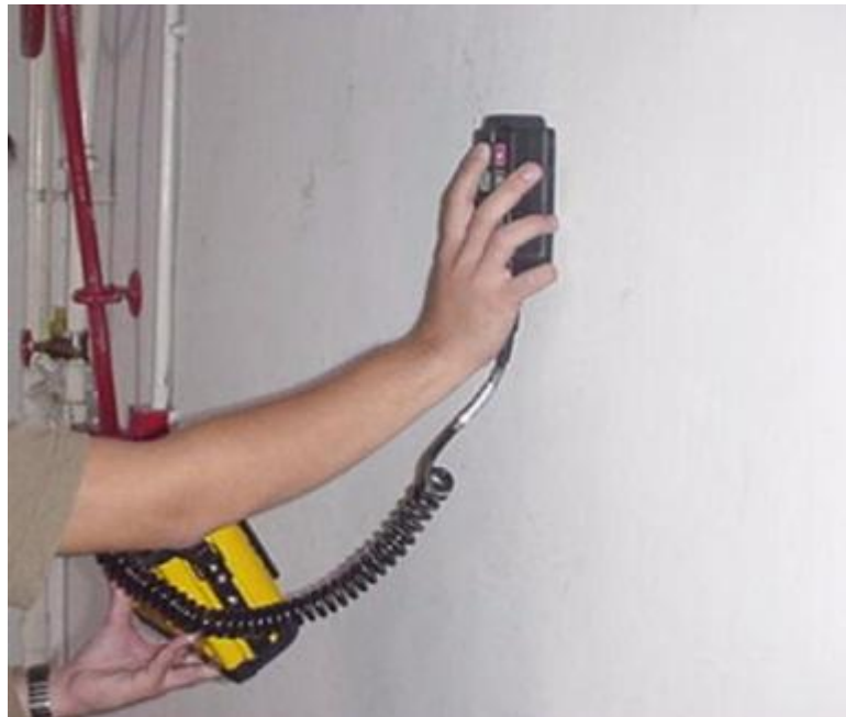
Figure 4.3: Scanned over the concrete surface
