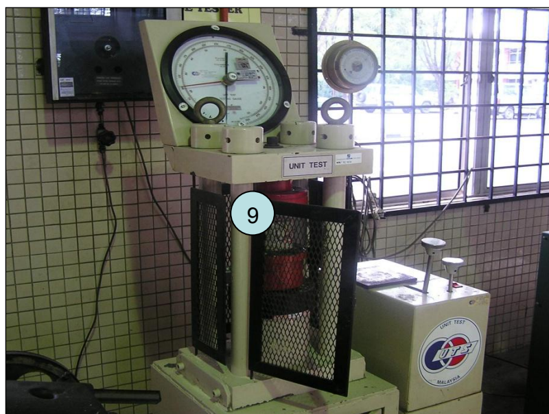
Figure 5.2: Compression Test Machine
