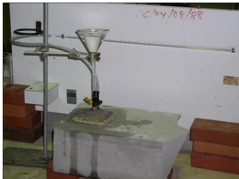
Figure 11.3: Complete set-up of ISAT test
