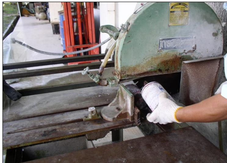
Figure 5.5: Grinding of specimen with grinding machine
