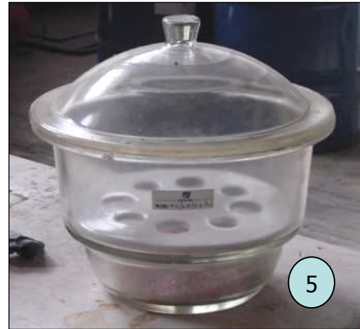
Figure 14.3: Sorption test apparatus
