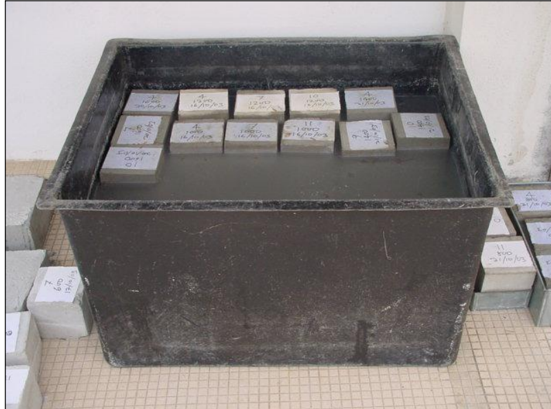
Figure 3.7: Store the specimen in water
