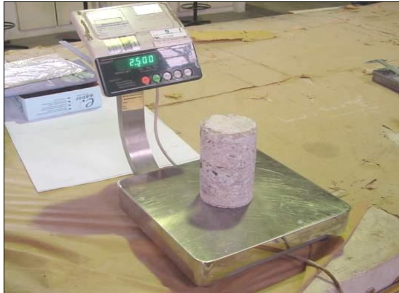
Figure 14.5: Weigh the specimen on a balance
