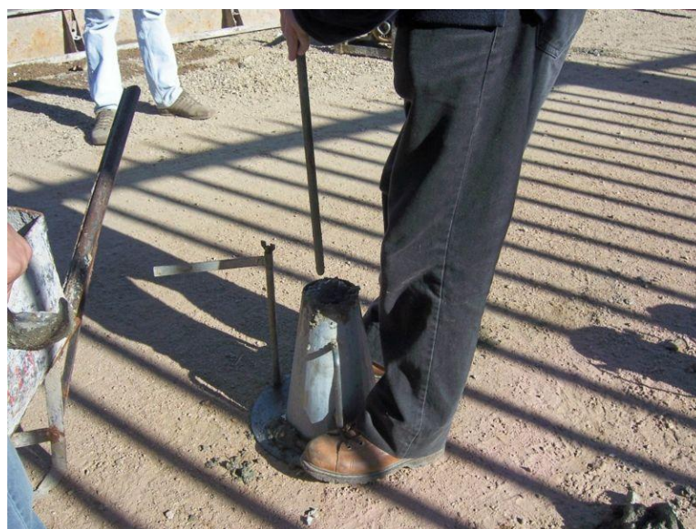
Figure 2.3: Hold the slump cone using 2 foot
