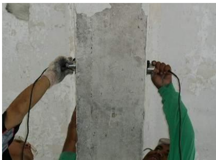
Figure 7.3: Arrangement of transducers for direct transmission
