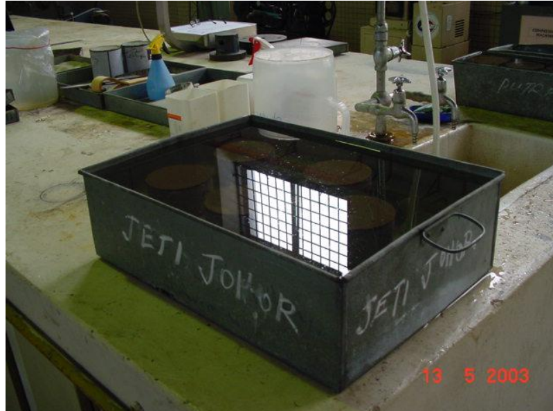
Figure 5.7: Store the specimen in water
