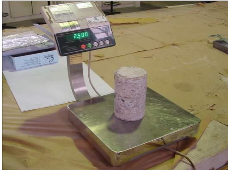
Figure 13.7: Weighing the specimen on a balance
