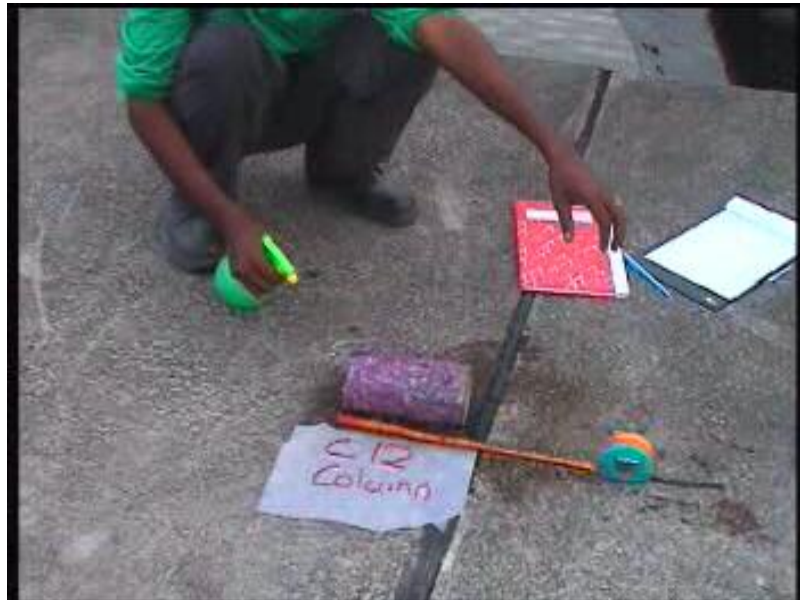
Figure 9.3: Spraying phenolphthalein solution on a core sample
