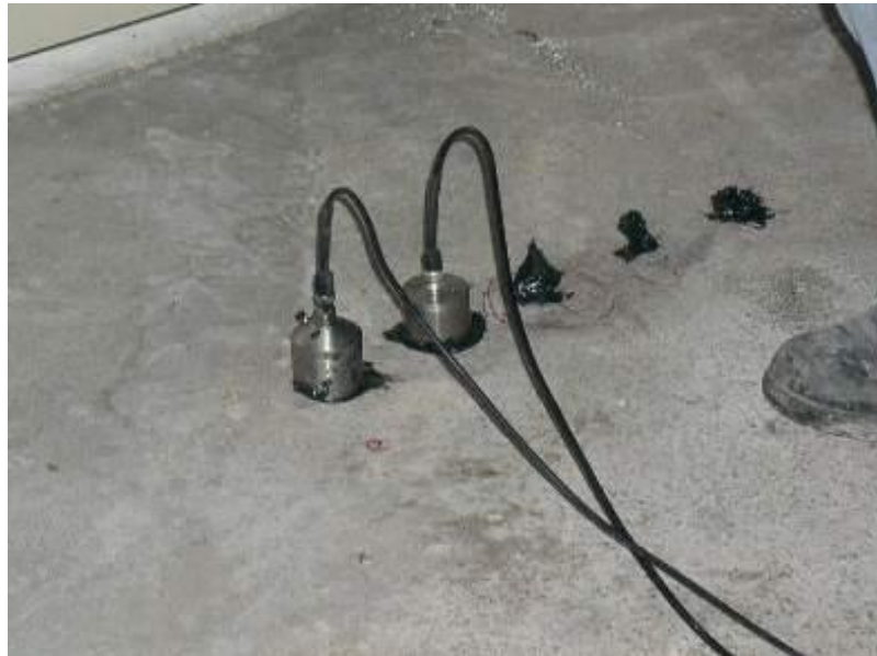
Figure 7.2: Applying coupling agent to transducers and structure surface
