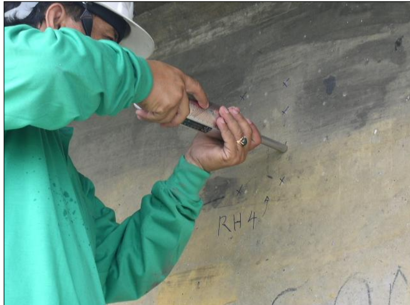
Figure 6.4: Holding the hammer perpendicularly to the test surface
