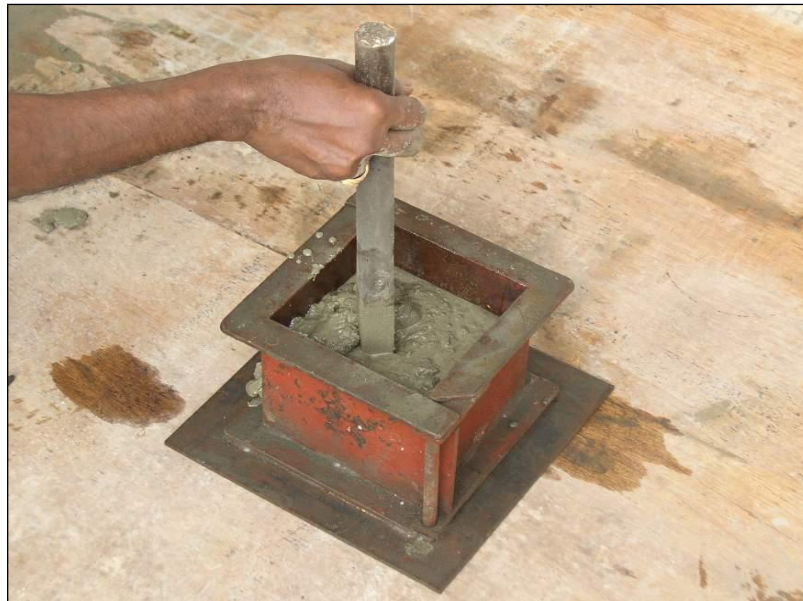
Figure 3.5: Compaction of concrete with a compacting bar.
