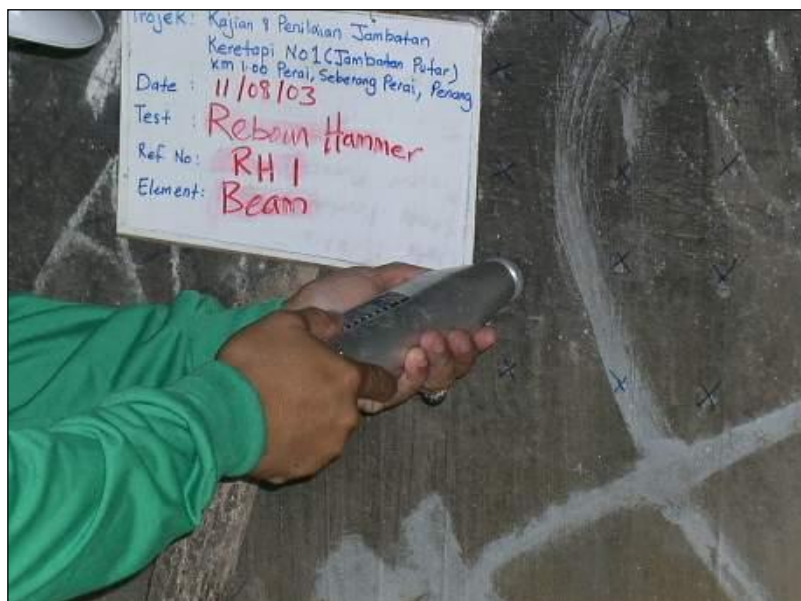
Figure 6.5: Pushing the hammer towards the test surface
