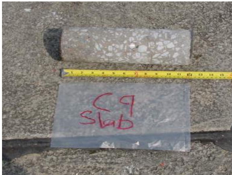
Figure 9.2: Core specimen ready for carbonation test
