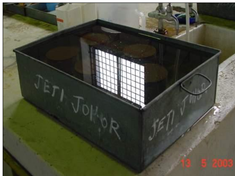
Figure 13.8: Immersion of specimen in water
