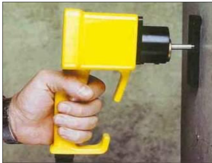
Figure 8.4: Measuring the exposed probe length
