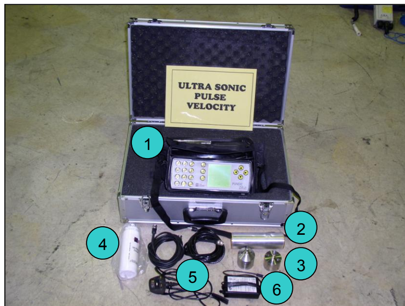
Figure 7.1: UPV test components
