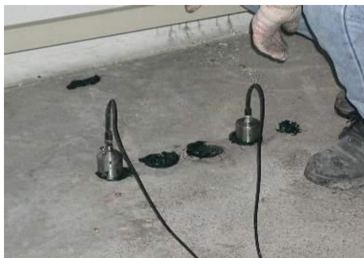
Figure 7.5: Arrangement of transducers for indirect transmission
