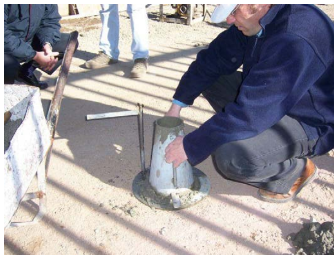
Figure 2.4: Slump cone slowly be removed
