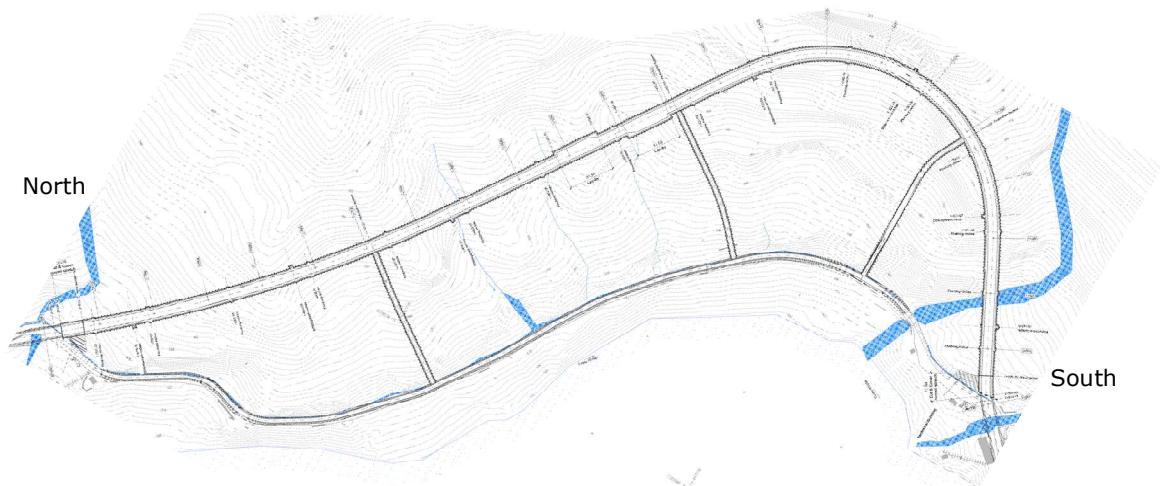
Figure 1: Horizontal alignment of the tunnel
