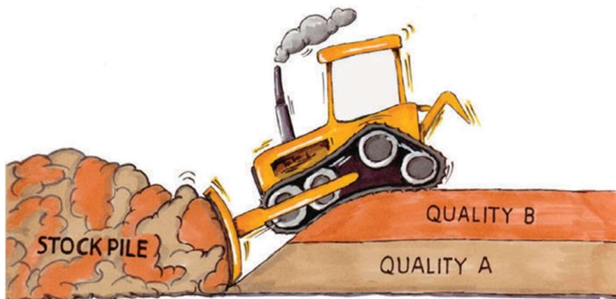
Figure 3-4 Non-recommended method for blending in borrow pit [11]
