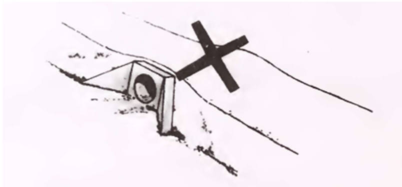
Figure 4-2: Avoid Hump at Culvert (Source: International Road Maintenance Hand Book Vol. II, Maintenance of Unpaved Roads, PIARC, Published by the TRRL, UK)
