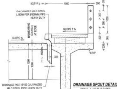
DRAINAGE SPOUT DETAIL SCALE - 1:40 @ A3 PAPER
