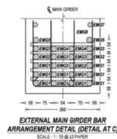
EXTERNAL MAIN GIRDER BAR ARRANGEMENT DETAIL (DETAIL AT C) SCALE: 1:10 @ A3 PAPER
