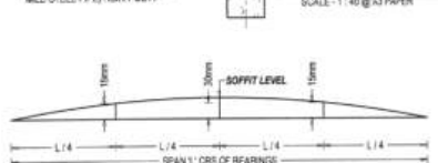
LONGITUDINAL CAMBER PROFILE TO BE GIVEN TO SOFFIT OF DECK SCALE - NON
