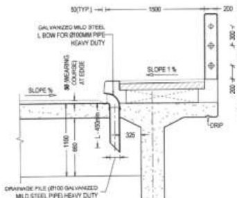
DRAINAGE SPOUT DETAIL SCALE - 1:40 @ A3 PAPER
