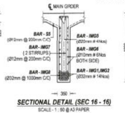
REINFORCEMENT DETAILS OF INTERIOR MAIN GIRDER - LONGITUDINAL HALF SECTIONAL VIEW SCALE - 1:100 @ A3 PAPER
