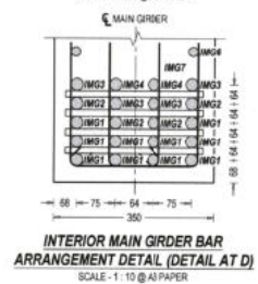
INTERIOR MAIN GIRDER BAR ARRANGEMENT DETAIL (DETAIL AT D) SCALE - 1:10 @ A3 PAPER
