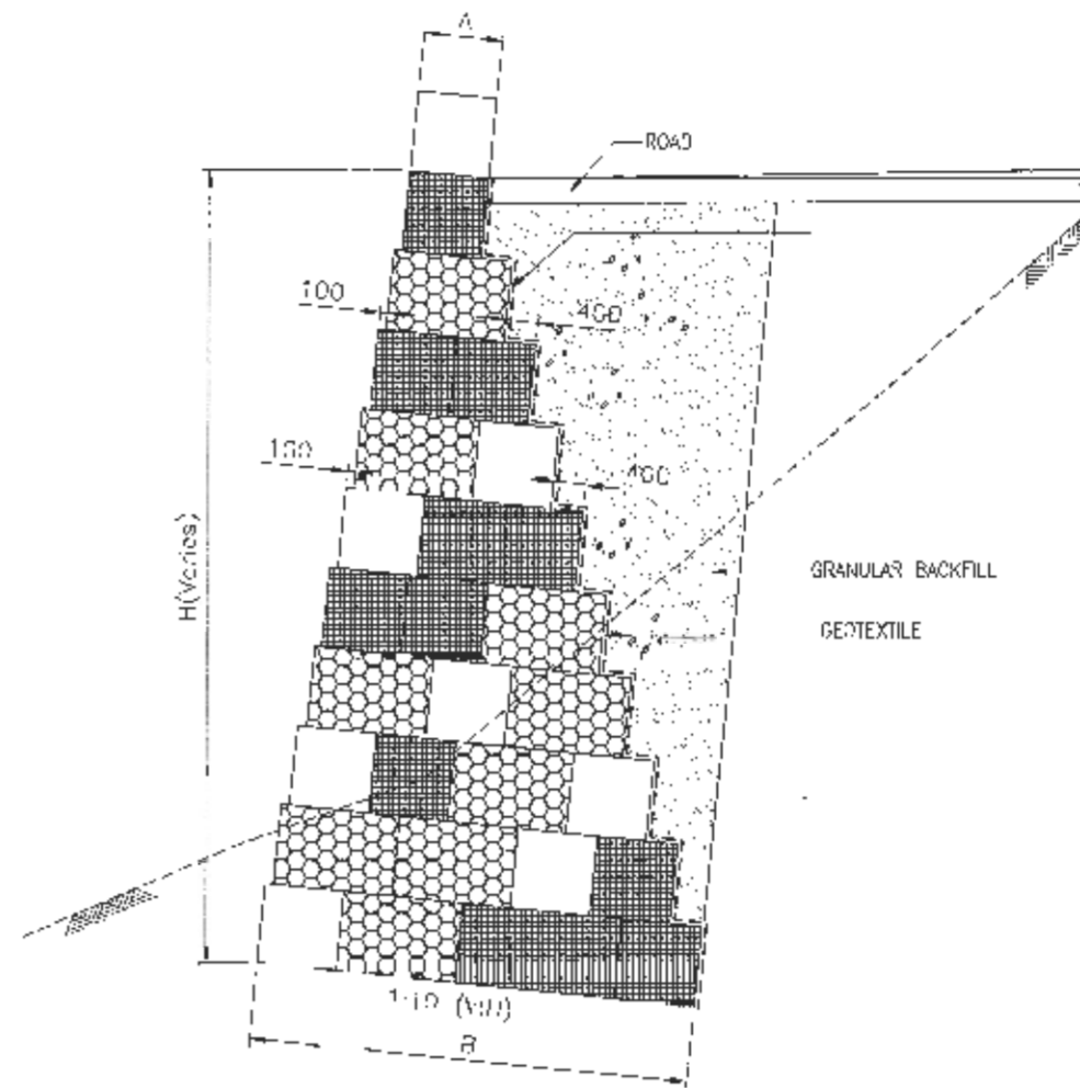
GRAVITY GABION WALL (BACK BATTER)
