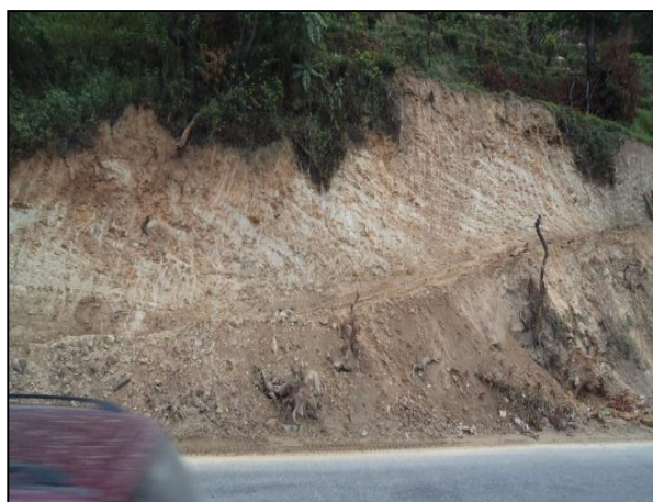
Outcrops of highly to completely weathered rocks of Sopyang Formation at Km 5+950
