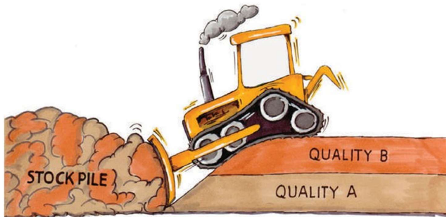
Figure 3-4 Non-recommended method for blending in borrow pit [11]
