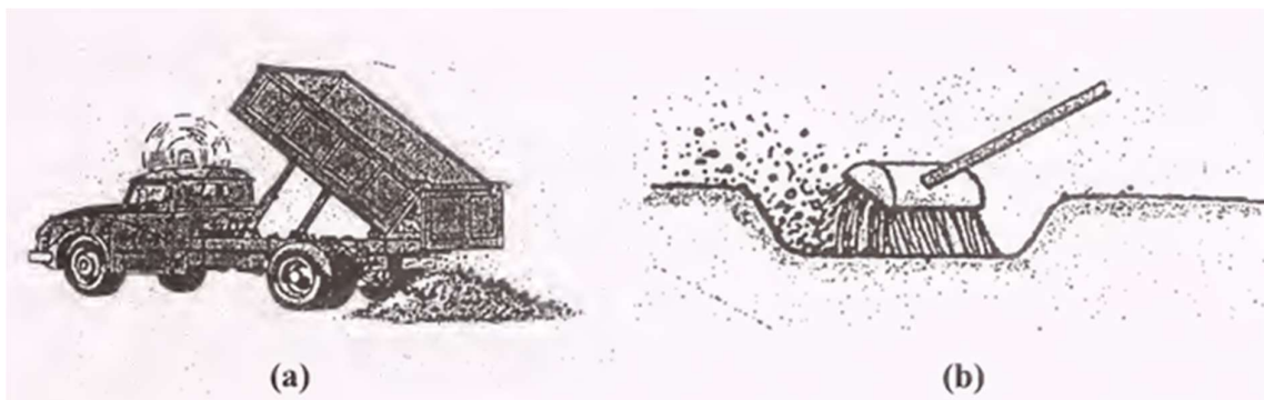
Figure 4-8:(a) Dump the material on the shoulder adjacent to location of patching work (b) Brush out any loose material or standing water (Source: International Road Maintenance Hand Book Vol. II, Maintenance of Unpaved Roads, PIARC, Published by the TRRL, UK)
