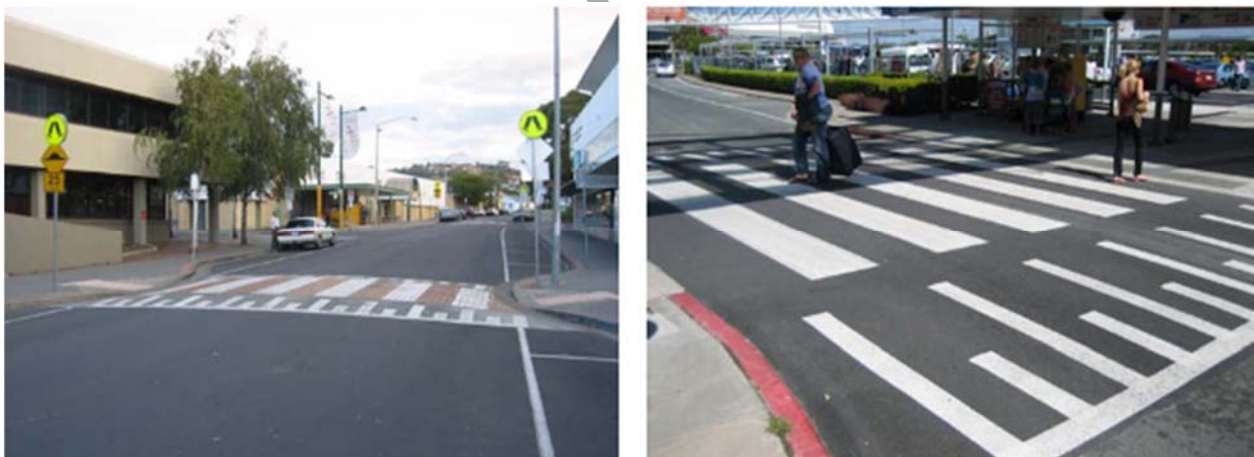
Figure 6.22: Raised Pedestrian Crossings
