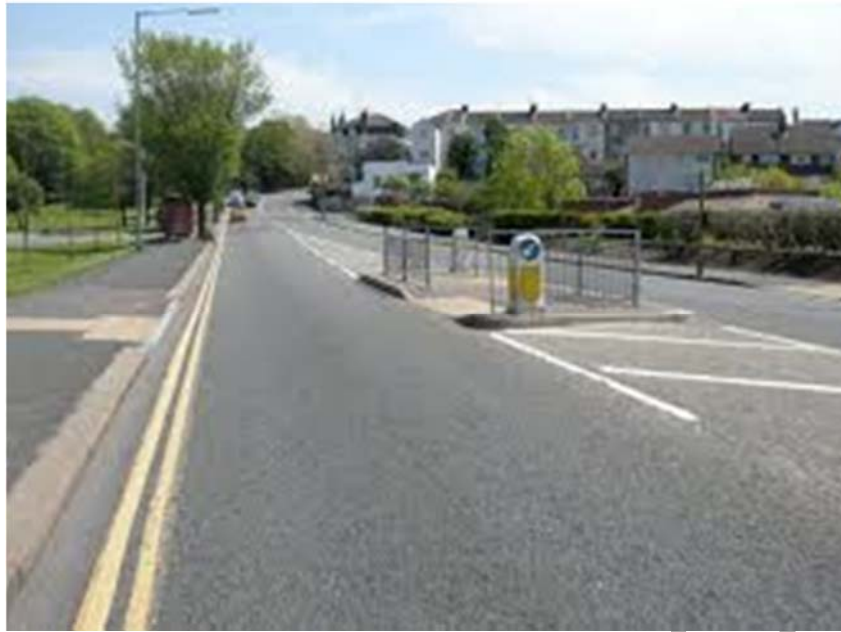
Figure 6.23: Two stage Crossings with Safety Cage
