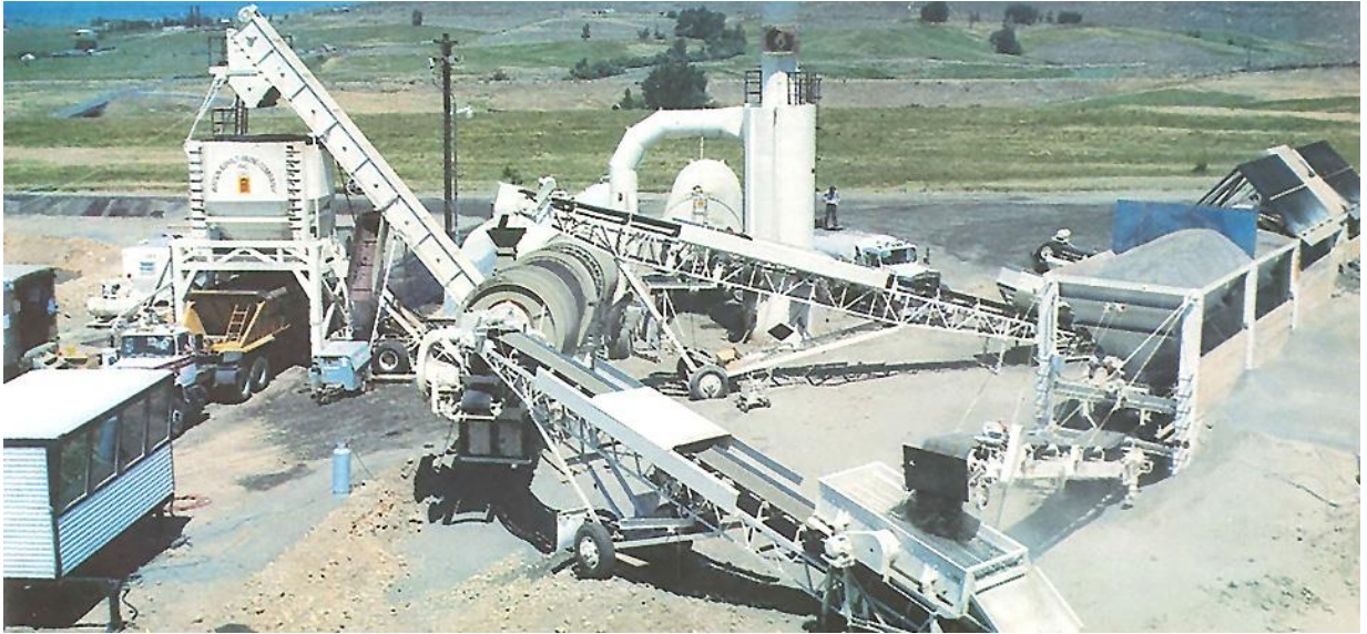
Figure 4.4 A typical parallel-flow drum-mix plant
