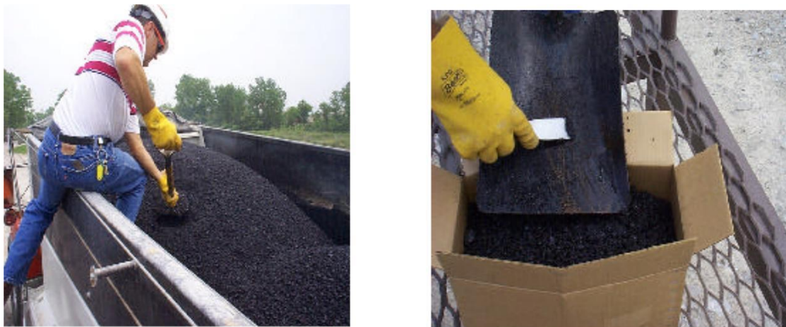
Figure 6.2 Sampling from a Truck Scraping Sample Off Shovel into Sample Box
