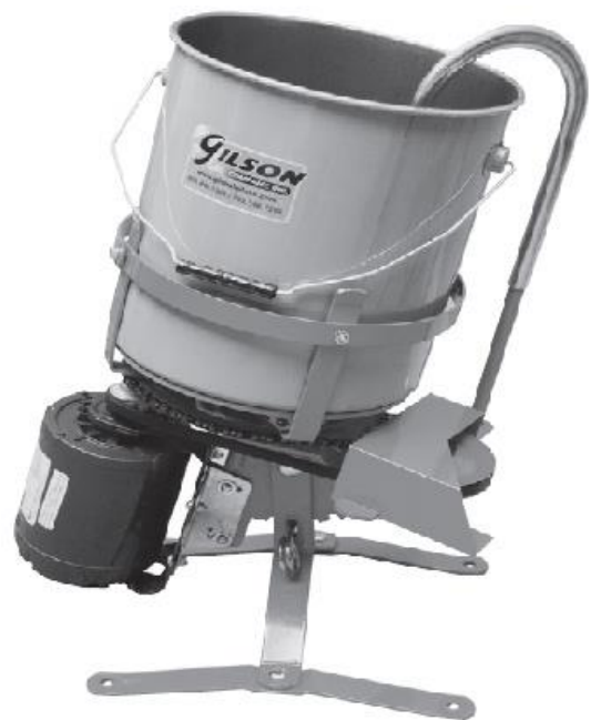
Figure 3.3 Planetary mixer with wire whips (Left) , a five-gallon bucket mixer (Right)
