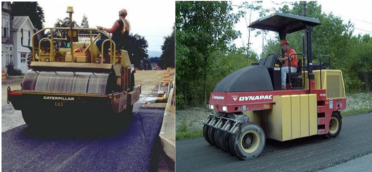
Figure 5.2 Vibratory roller (Left) & Rubber tired roller(Right)
