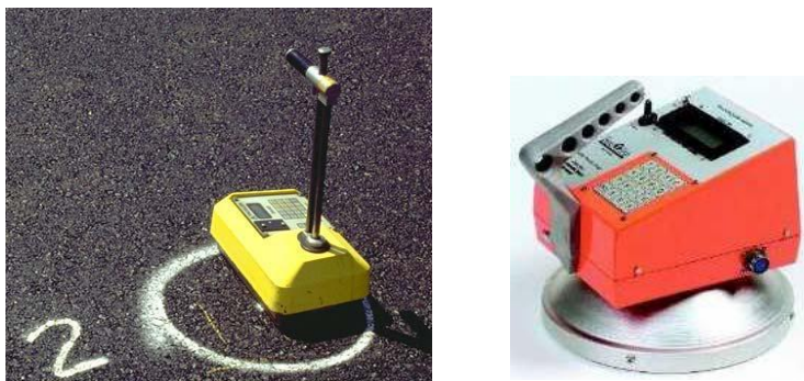
Figure 6.5 Nuclear density gauge (Left) Non-nuclear density gauge(Right)
