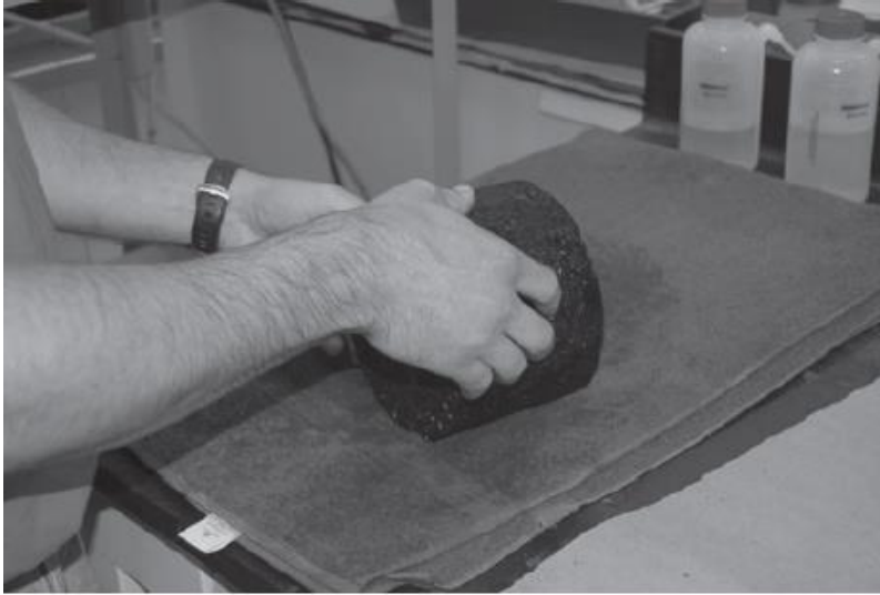
Figure 3.7 Determination of SSD mass of specimen
