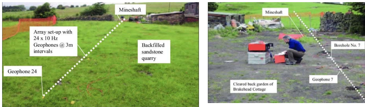
Figure B-13A: Procedure for Micro Tremor Survey example
