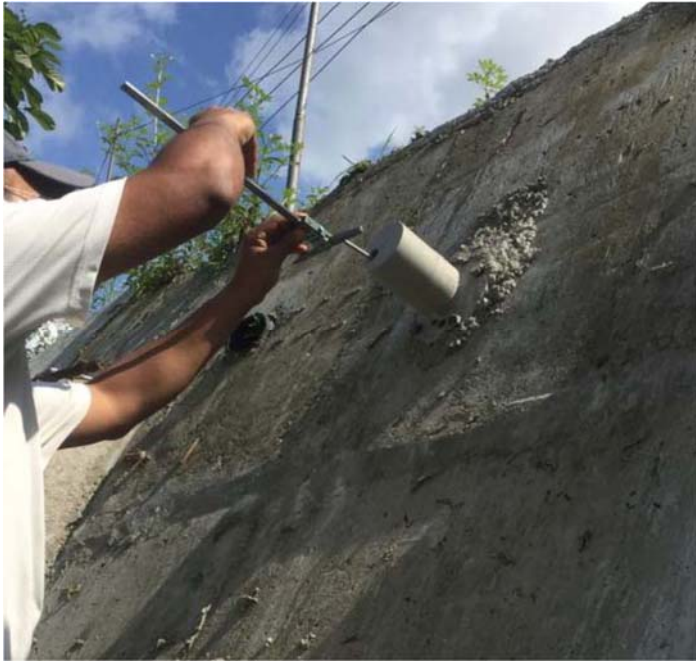
Extensometer test at km 26 of Narayanghat Mugling Road
