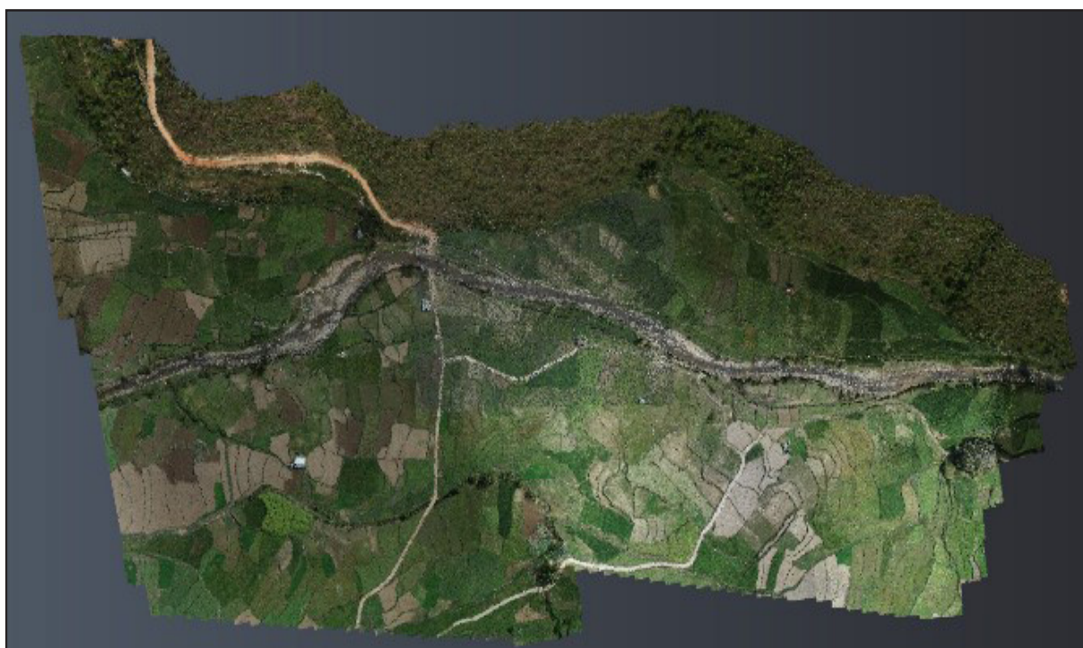
Fig. 5: Topographic details, generated from a drone survey
