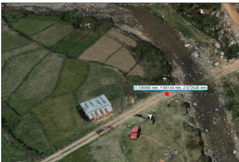
Fig. 3: Accurate Point Cloud Plan View showing the X, Y, and Z data and Topographic Visualization
