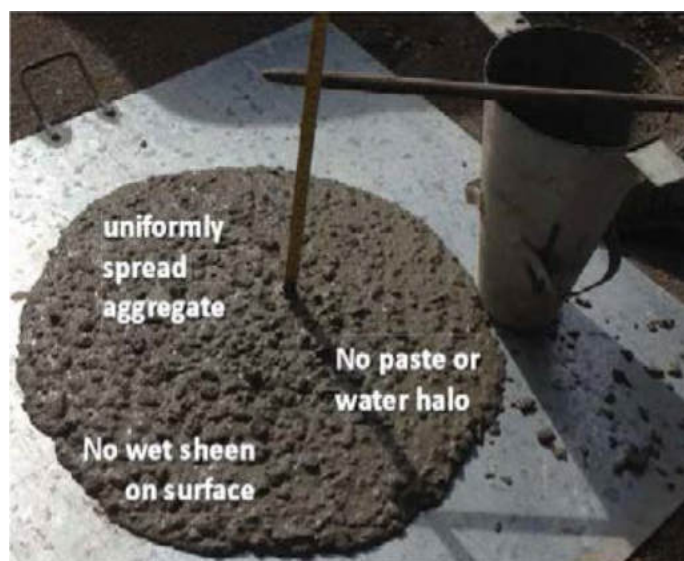
Fig.3- Slumped concrete of Visual Stability Index =0
