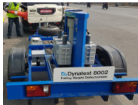
Fig1: Falling Weight Deflectometer (FWD)
