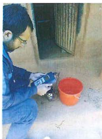
Onsite bacterial Culture in Del Agua Kit (left) and Onsite measurement of pH, conductivity and temperature (right)
