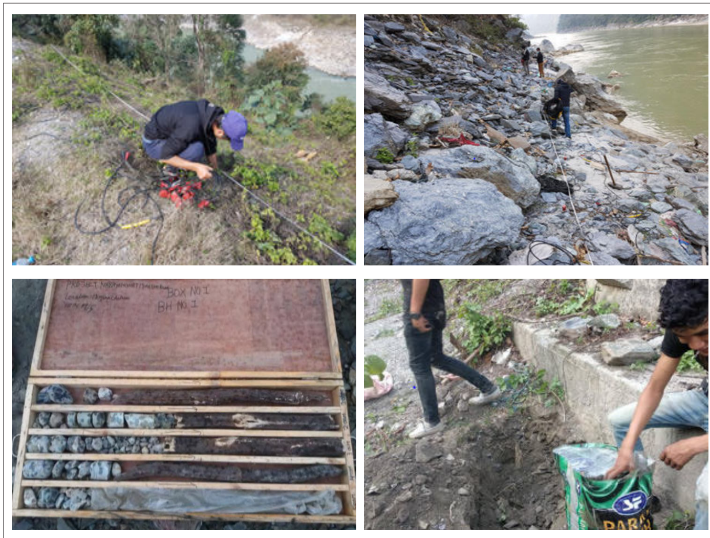
Fig. 5.1 : Geotechnical Investigations performed at Chainage 17+025 km, Chitwan.
