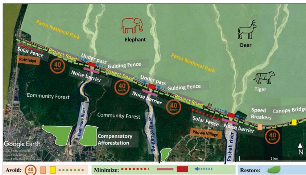
Figure 1.5: Project Site and Landscape with Application of the Mitigation Hierarchy
