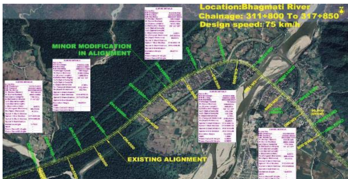
Figure 8.5: Alignment along Bagmati River Bridge and Approaches
