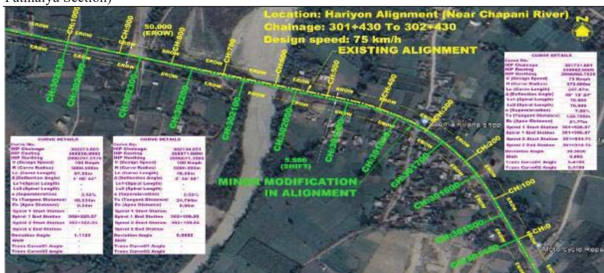
Figure 8.4: Minor Realignment at Hariyon
