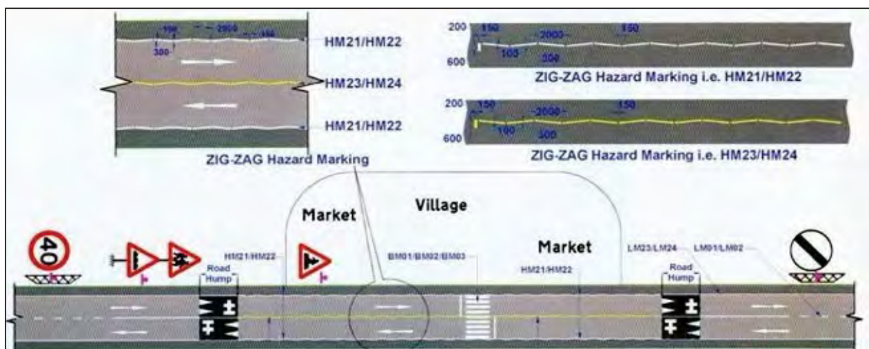
Figure 4: Zigzag Hazard Marking (Source: IRC-35)
