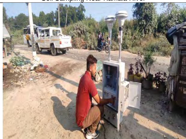
High Volume Air Sampler installation at Dudhaura
