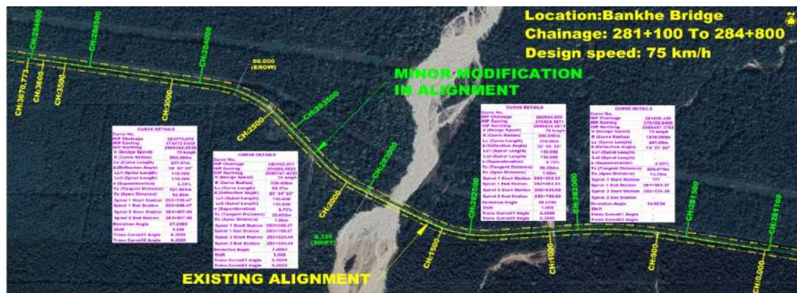
Figure 6-5: Alignment at Approaches of Bankhe Bridge
