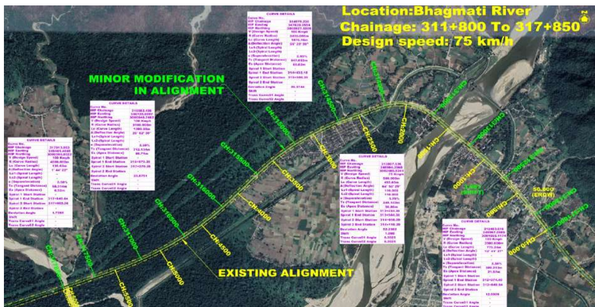
Figure 6-3: Alignment along Bhagmati River Bridge and Approaches
