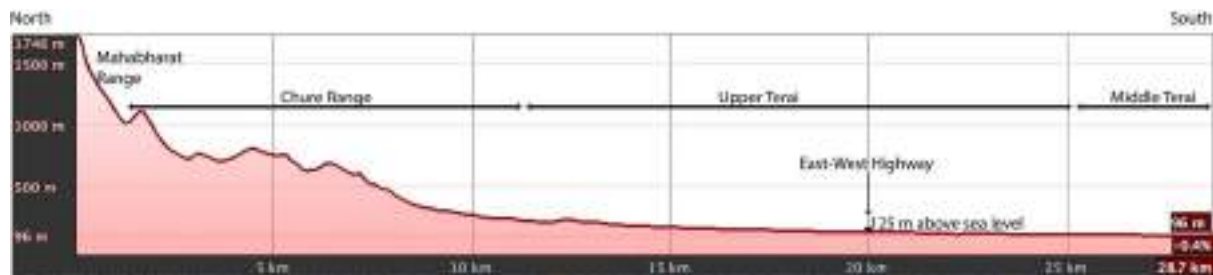
Figure 6.1: General north-south topographical profile across the East-West Highway, which shows the various geomorphic zones
