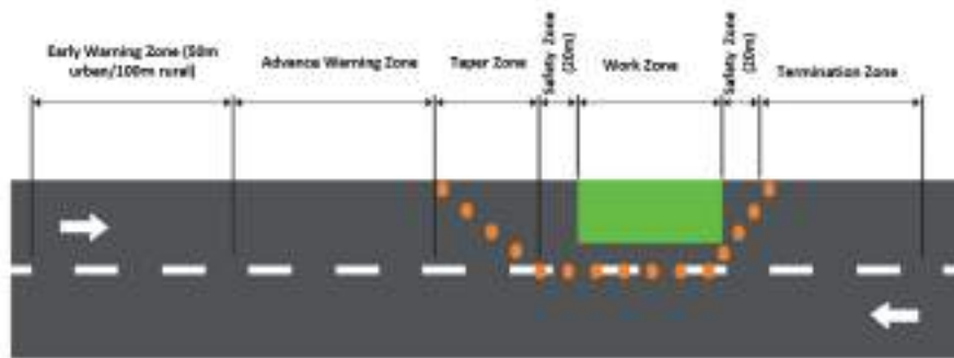
Figure 11.16 : The Six Zone Concept for developing Temporary Traffic Management Plan 11
