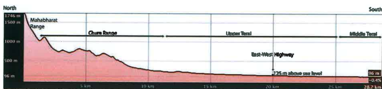
Figure 16: General north-south topographical profile across the East-West Highway, which shows the various geomorphic zones
