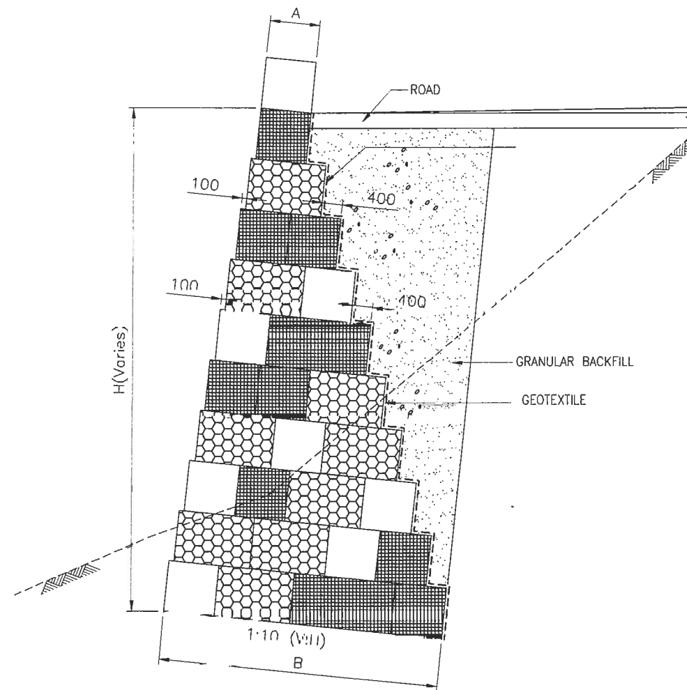
GRAVITY GABION WALL (BACK BATTER)
